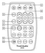
When it comes time to replace the remote's battery, use only a major brand name 3V Lithium battery compatible with model CR2025. Slide the battery cover off and install the new battery with the positive "+" side facing up.
